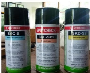
Gambar 3.3 *Liquid Penetrant (Cleaner, Penetrant & Developer)*
