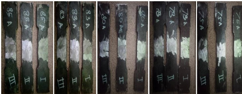
Gambar 4.2 Spesimen Uji Tarik ASTM E8
