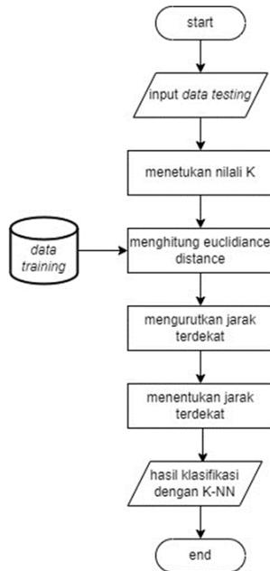
Gambar 1. Flowchart Algoritma K-NN
